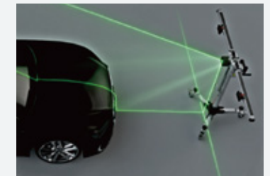
High Accuracy (Five-line laser and cross laser)
